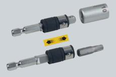
For use with 1/4" sockets and 1/4" hexagon standard bits (6.3mm) on cordless screwdrivers and electric drilling machines. Choice between the two options simply by sliding the sleeve.
