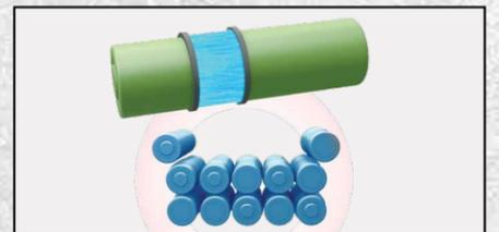
Each cell is wrapped with a temperature controlling material that keeps cells cool to provide better performance.
